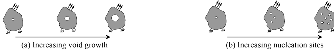
Figure 3.2. Damage framework with limiting cases of single void growth in (a) and by void nucleation.
